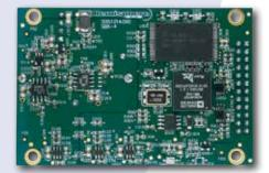
Provide a reliable source of differential corrections with the SBX- $4^{\text{TM}}$  radiobeacon board that augments a separate GPS receiver with free accuracy-improving correction data from networks of beacon stations located throughout the world.
